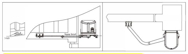
Notice: The front bracket and motor must be in same level!
